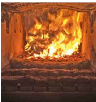
Magno-VR with forward flat bed step grate
