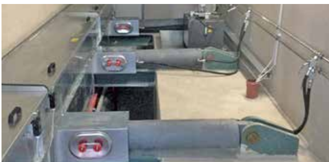
Solid hydraulic cylinders to enable movement of moving floor
