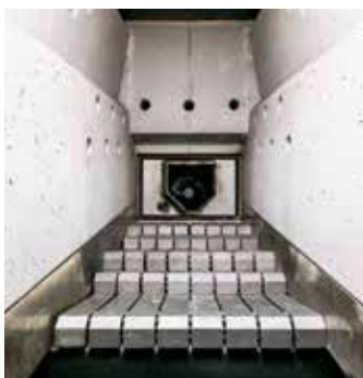
Magno-VR with forward flat bed step grate
