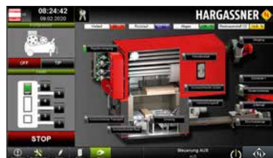
Function & relay test for all sensors and motors
